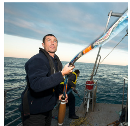
Mountjoy in Kaikoura operating a seismic streamer used for the 3D survey. Credit: Dave Allen, NIWA.
