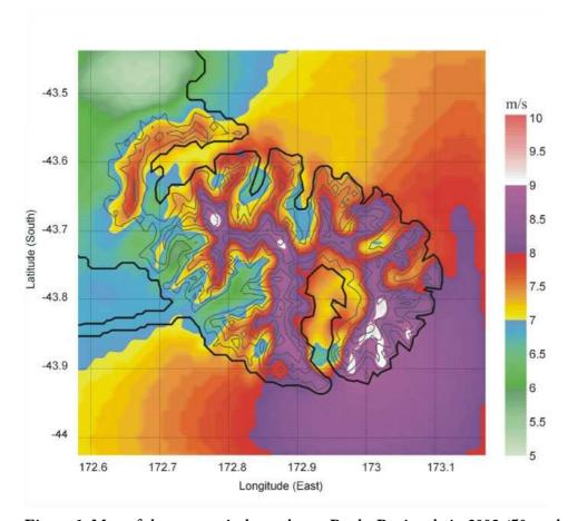
Figure 1. Map of the mean wind speed over Banks Peninsula in 2002 (50 m above ground at a resolution of  $800 \, \mathrm{m}$ ), from the collaboration between Canterbury University and Connell Wagner.
